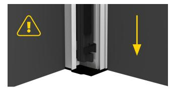
The PVC-side channel extends from the aluminium side channel. If you shorten the aluminium side channel, you need to take into account the same overlength for the PVC side channel.
